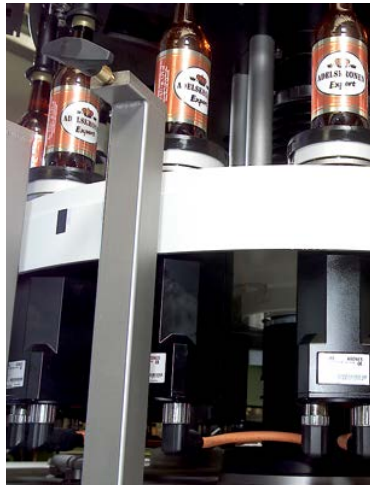
Container table with servomotors, protection type IP65
